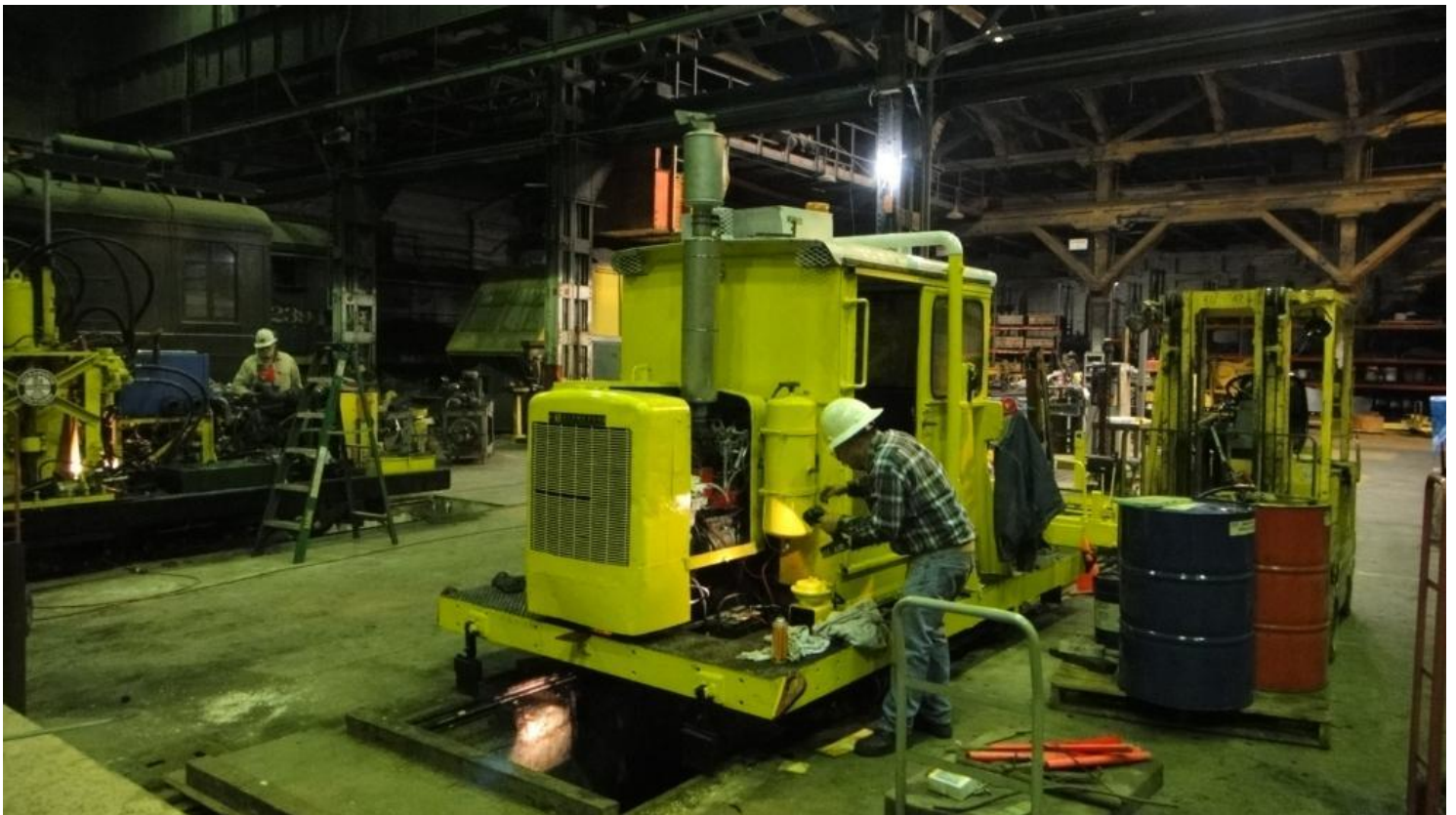
Hydraulic tank fill, diesel added, the Kalamazoo fired right up and is running. In no time, this machine will be out on the line
