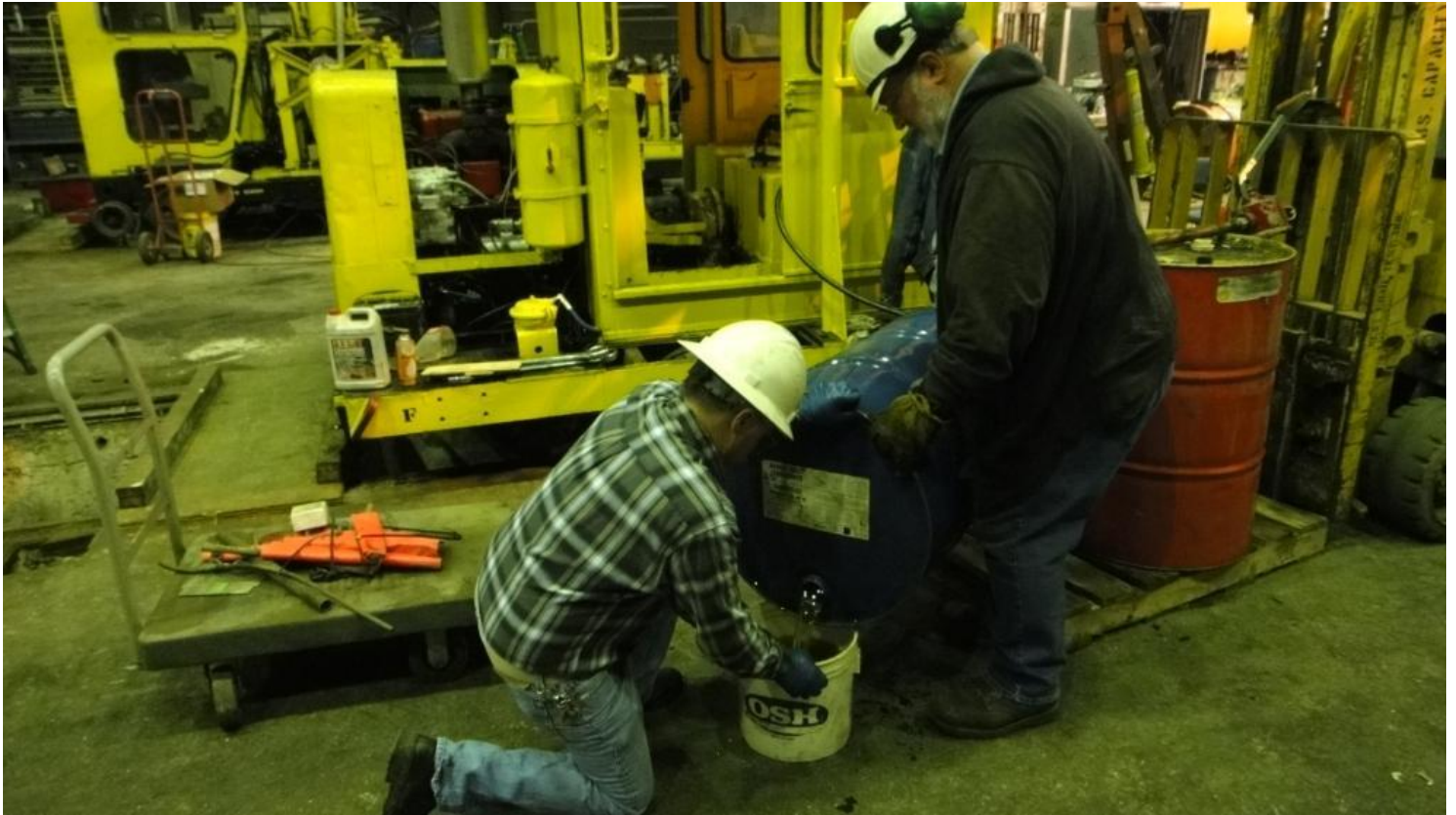
Frank pours hydraulic from the 55 gallon drum which Mike H. will then add to the Kalamazoo's hydraulic tank
